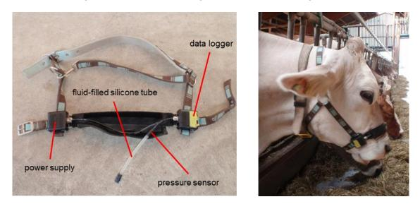
FIGURE 1: RumiWatch noseband sensor containing a fluid-filled silicone tube with built-in pressure sensor and two electronic units
